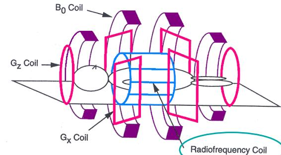
Simplified Drawing of Basic Instrumentation.
