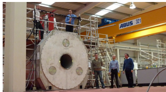
The 11.7 T MR magnet with members of the MRI team at Agilent's Magnet Technology Center in Yarnton, UK (from left to right): Darren Houlden, Andrew Winter, Paul Johnson, Nigel Haynes and Alistair Courtney.
