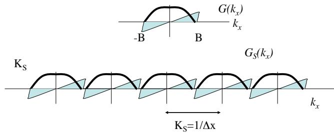
To avoid overlap, we require that  $1/\Delta x > 2B$  or  $K_S > 2B$  where  $K_S = 1/\Delta x$  is the sampling frequency
